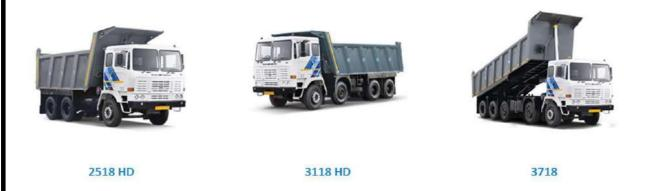
These three products full demand product in Mining and Construction segment, where **2518 HD** is a Tipper truck, Gross Vehicle Weight is 25ton, Power: 180 HP @ 2500 rpm Torque: 660Nm @ 1200~1900 rpm.
